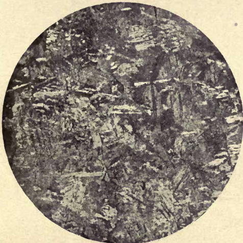
Fig. 25. \times 10 Alloy 68. Cu 60.4 Slowly cooled in Sn 6.0 furnace. Zn 33.6 \alpha + \gamma eutectoid.
